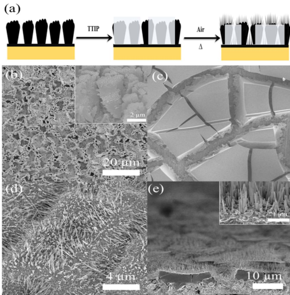
**Figure 8. (a) Diagram showing the multistep strategy that convert CuS dendrites into hybrid TiO<sub>2</sub> blocks covered with CuO nanorods, SEM images of (b) CuS dendrites, (c) CuS dendrites covered with Ti precursor block after drying, (d) TiO<sub>2</sub> blocks covered with CuO nanorods, and (e) cross section of the TiO<sub>2</sub> blocks covered with CuO nanorods.**
