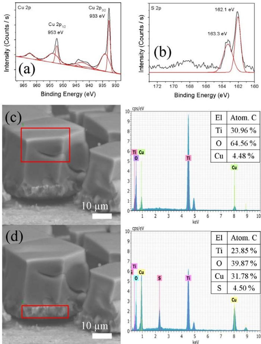
**Figure 9.** XPS spectra of CuS dendrite showing (a) Cu 2p and (b) S 2p regions. Cross-sectional SEM and EDS data of (c) upper side and (d) down side dried CuS dendrite covered with Ti precursor blocks.
