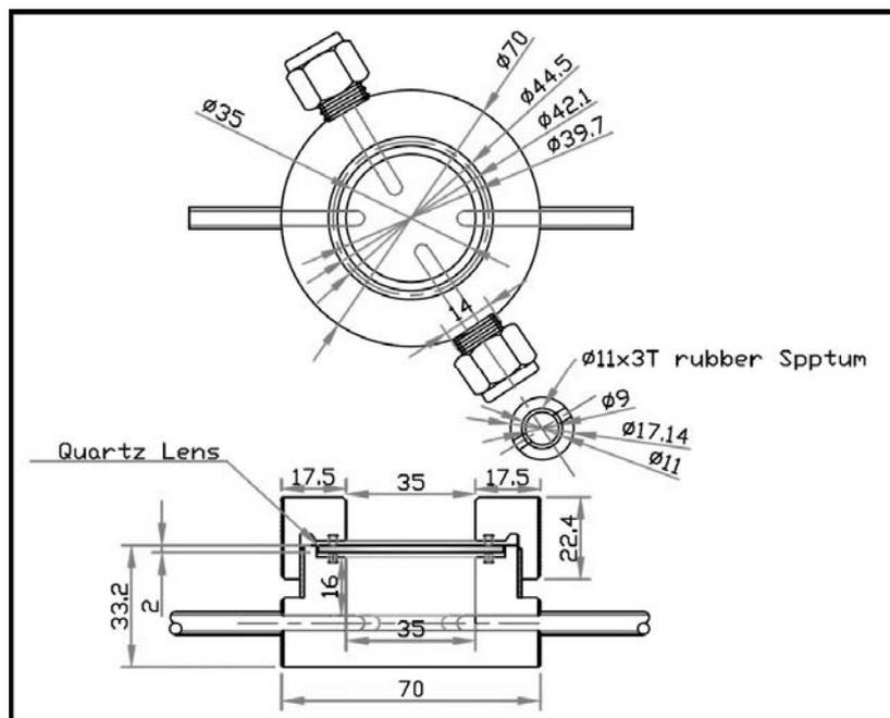
**Figure 6. Design of photoreactor used for CO<sub>2</sub> photoconversion.**
