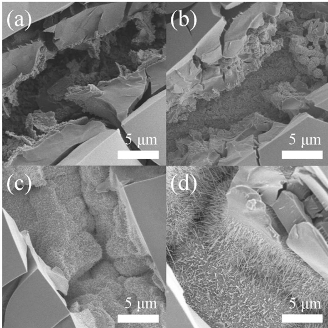
**Figure 10. FESEM images of TiO<sub>2</sub> presursor-CuS dendrites annealed for 1 hour at (a) 100 °C, (b) 200 °C, (c) 300 °C and (d) 400 °C.**
