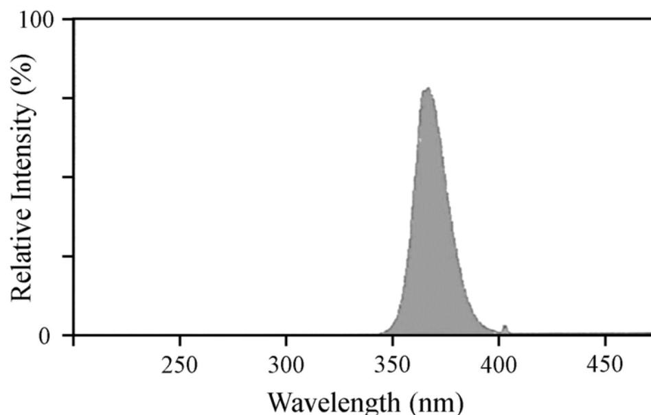
**Figure 7. Spectral chart of UVB lamp (( $\lambda_{\text{max intensity}} = 365 \text{ nm}$ , UVP Inc. UVGL-58) referred to UVP Inc.**
