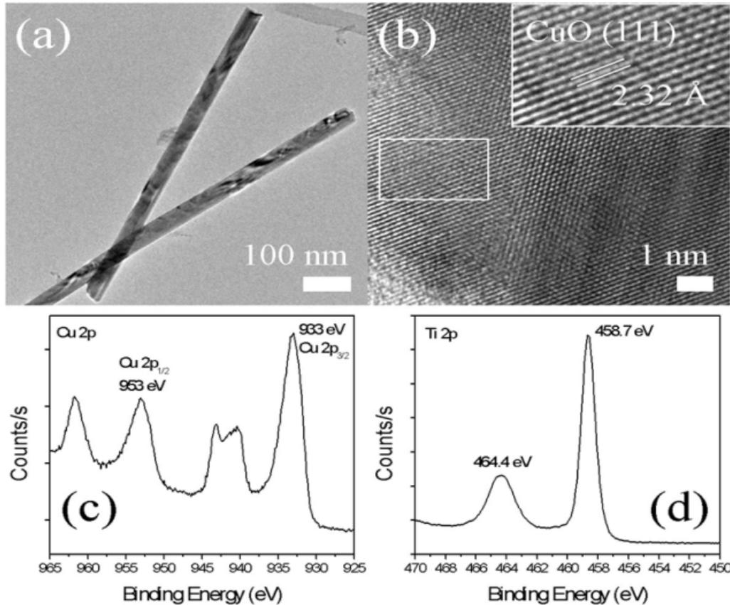
**Figure 11. (a) TEM of CuO nanorods, b) HRTEM of CuO nanorods, and XPS spectra of c) Ti 2p and d) Cu 2p regions, respectively.**
