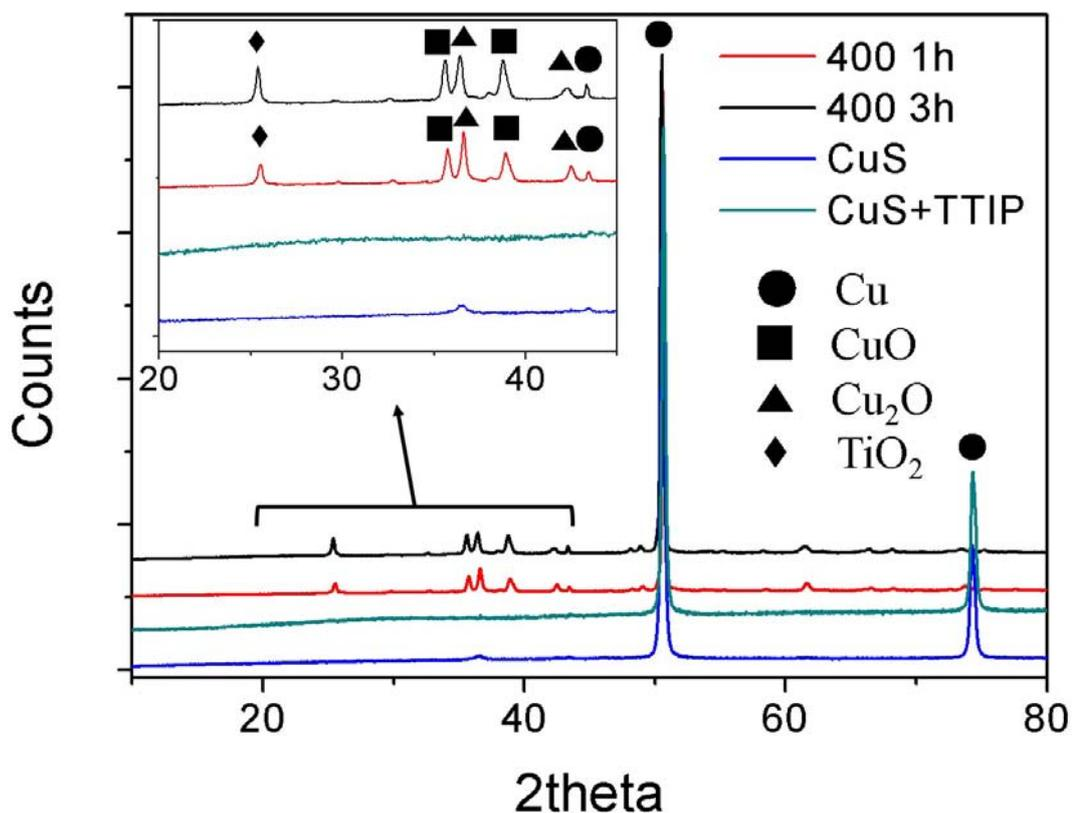
**Figure 12. Powder XRD of CuS dendrite (blue), Ti precursor on the CuS dendrite (green), TiO<sub>2</sub> block-CuO nanorods annealed for 3 hours (black) and 1 hour (red) at 400 °C.**
