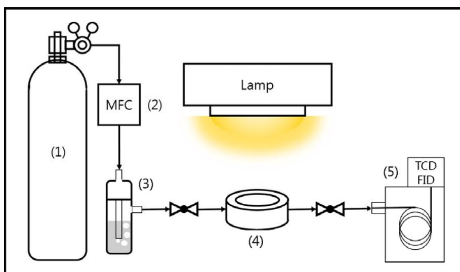
**Figure 5. The schematic representation of the experimental setup for CO<sub>2</sub> photoreduction comprising of (1) CO<sub>2</sub> gas Cylinder, (2) Mass Flow Controller, (3) Gas bubbler containing deionized water, (4) Photoreactor for conversion of CO<sub>2</sub>, (5) Gas Chromatography unit**
