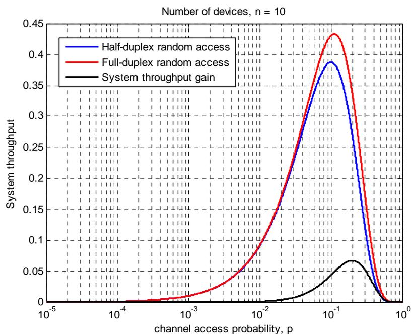
Figure 9. System throughput for number of devices and access probability in FD and HD communication
