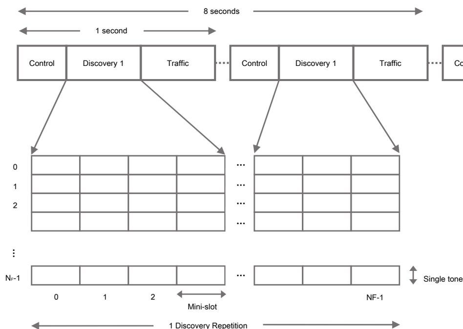
Figure 5. Device discovery in timing structure
