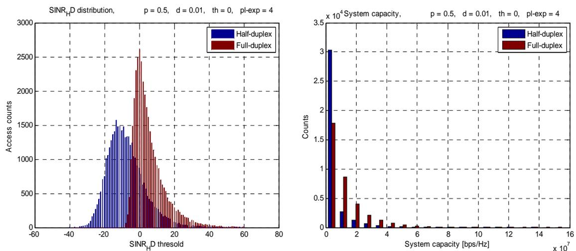
Figure 12. SINR distribution and system capacity for FD and HD
