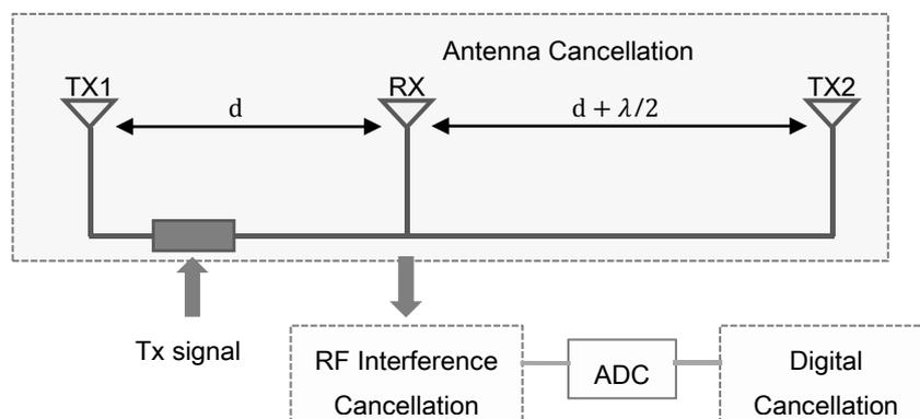
Figure 2. Block diagram of existing full-duplex design with three cancellation techniques.
