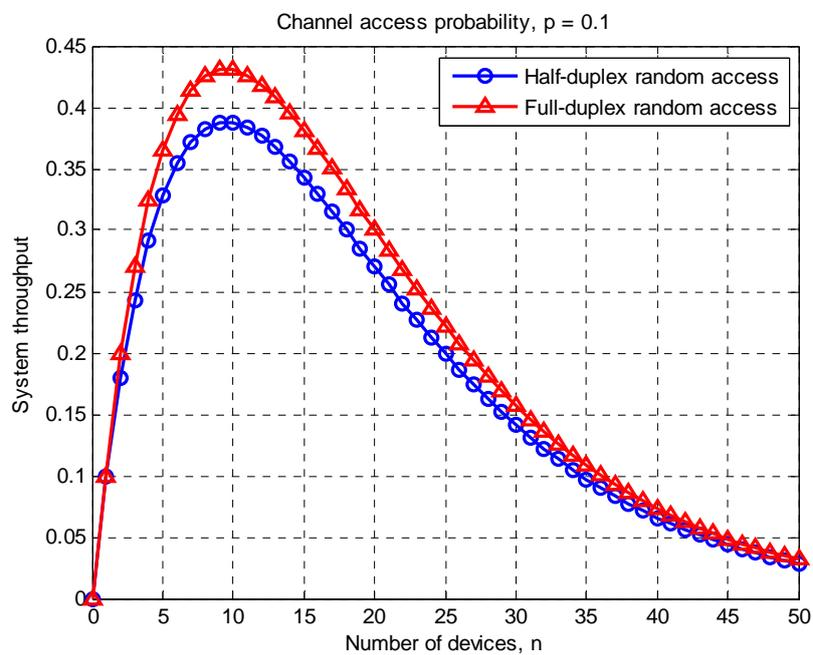
Figure 10. System throughput for the number of devices using the FD random access
