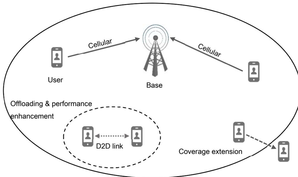
Figure 4. Device-to-device communication
