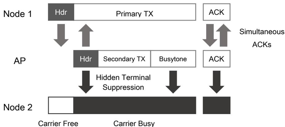
Figure 3. Full-duplex MAC protect primary and secondary transmission from hidden terminal losses.
