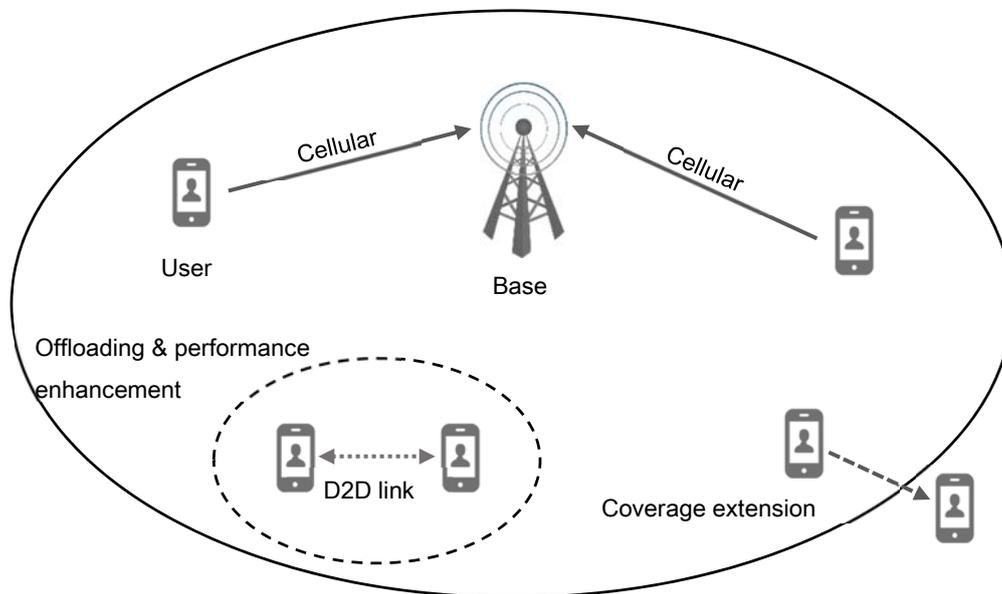
Figure 4. Device-to-device communication
