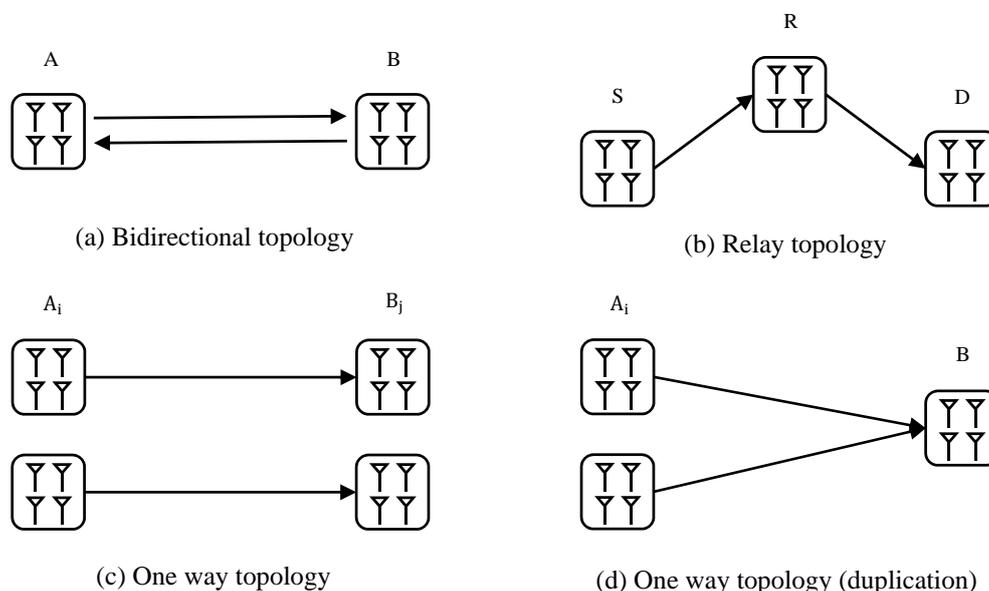
Figure 8. Transmission topologies for two active devices
