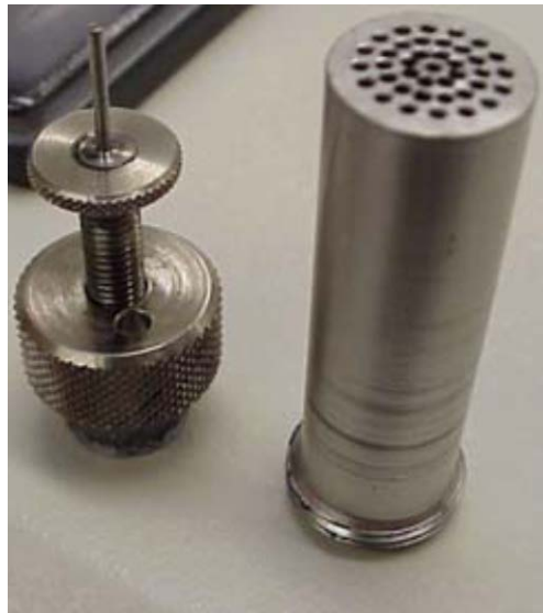
Fig. 3. Fiber chamber SH0620 (Krüss, Hamburg, Germany)
