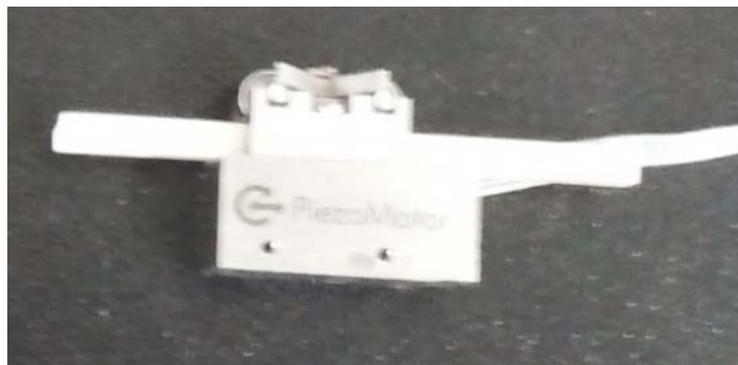
**Figure 3-2. The PZT motor.**
