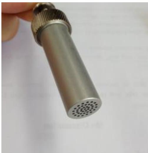
**Figure 5. Fiber chamber SH0620 (Krüss, Hamburg, Germany).**
