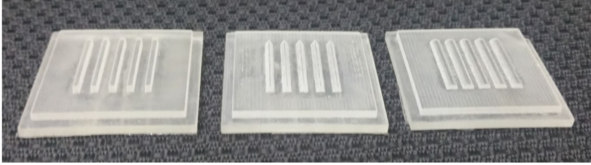
Fig 3.3.2 Optical image of the three different textures. The textures were designed to be removable and the textures were mounted on a linear stage for sliding experiments
