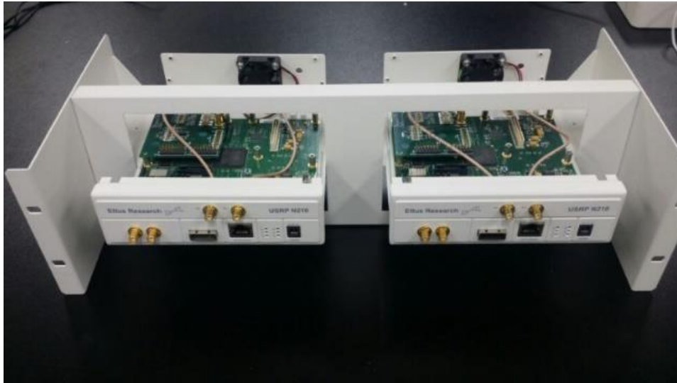
Figure 4.3 Software defined radio USRP N210 equipped with Basic Tx / Rx daughterboard
