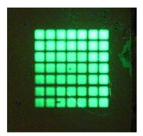
Fig. 5. Excitation characteristics of the P22 green phosphor using the  $\mbox{Pt}/\mbox{Ti}$  OPPS field emitter.
