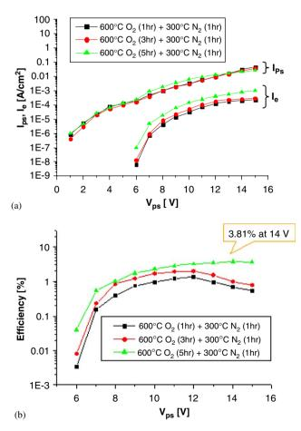
Fig. 3. Effect of thermal annealing time on (a) the driving current  $I_{ps}$  and emission current  $I_e$ , and (b) the emission efficiency of the Pt/Ti OPPS field emitter.
