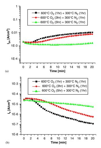
Fig. 4. Time dependent variation of the field emission characteristics of the OPPS field emitter.
