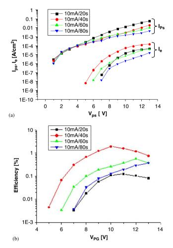
Fig. 2. Change of (a) driving current  $I_{ps}$  and emission current  $I_e$ , and (b) efficiency at various oxidation times.
