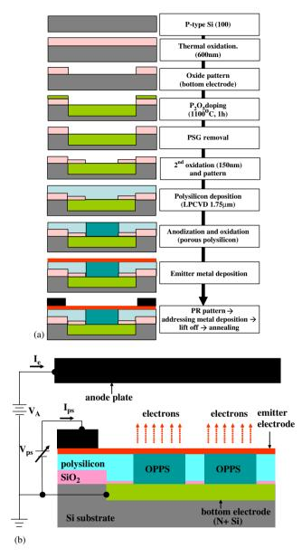
Fig. 1. (a) Fabrication of an OPPS field emitter and (b) cross-sectional view of the OPPS field emitter and the electrical connection for the analysis of its field emission characteristics.
