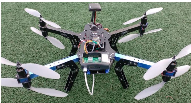
Figure 5.2. 3DR X8+ drone used for experiments.
