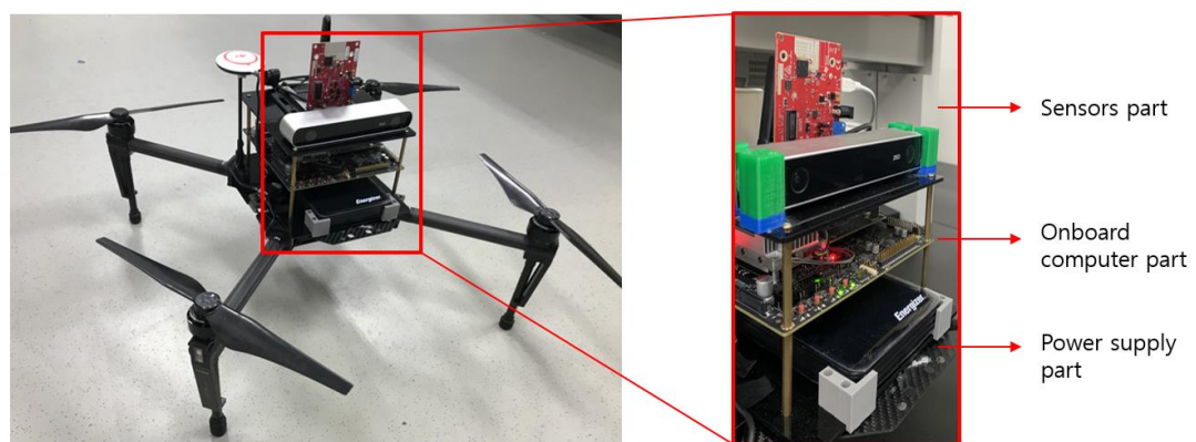
Figure 2. Three layers of plate manufactured separately and mounted on top of M100
