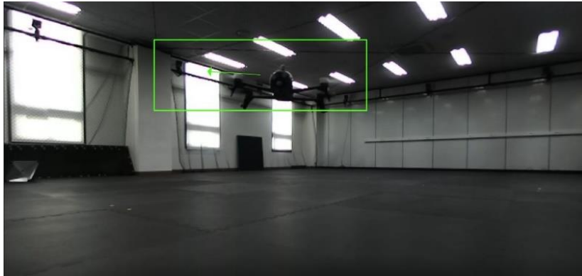
Figure 13. Experiment 1) Performance verification experiment about integration of YOLO drone detection system and SORT tracking algorithm
