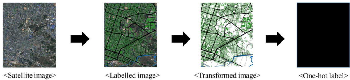
Fig. 15. The process of making the ground truth. The dataset covers an area of 551 \text{ km}^2 and is randomly divided into an area of 486.5 \text{ km}^2 for training and 64.5 \text{ km}^2 for testing. All the data were divided into multiple images with the pixel size of 224 \times 224 , of which 72,400 images were assigned to the training set and 9,600 to the test set.
