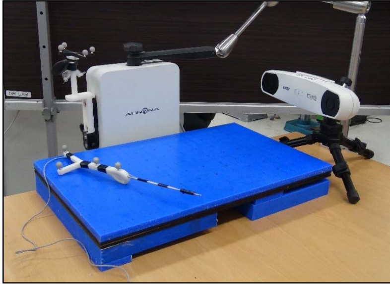
Figure 3.1 Experimental setup for collecting measurements from an EMTS and an OTS.
