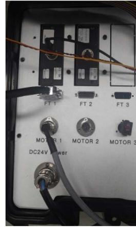
**Figure 3-3. Control box of the hand robot**
