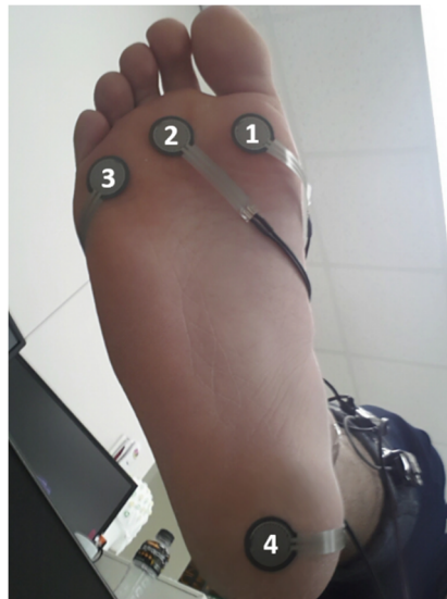
Figure 10. FSRs on foot. 1: First metatarsal, 2: Between second and third metatarsal, 3: Fifth metatarsal, 4: Heel
