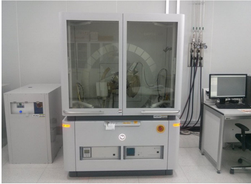
Figure 4.1: X-ray diffractometer (Empyrean PANalytical) in DGIST Fab.
