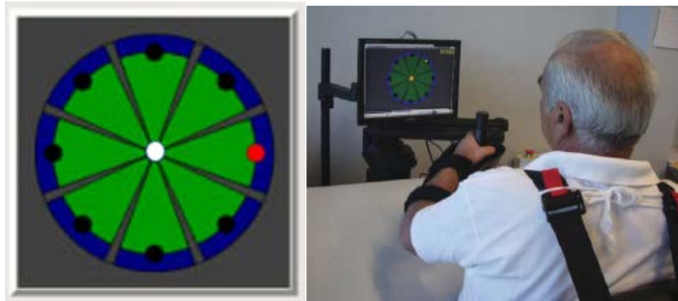
Fig 1. (a) The green clock Task. White circle is start location and red circle is target location. Target appears clockwise from 12'o clock direction. (b) The green clock task with MIT-MANUS
