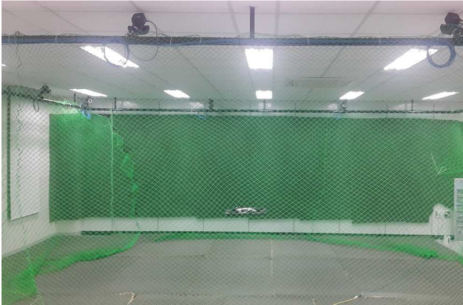
Fig. 4.3. VICON system with a hovering drone.
