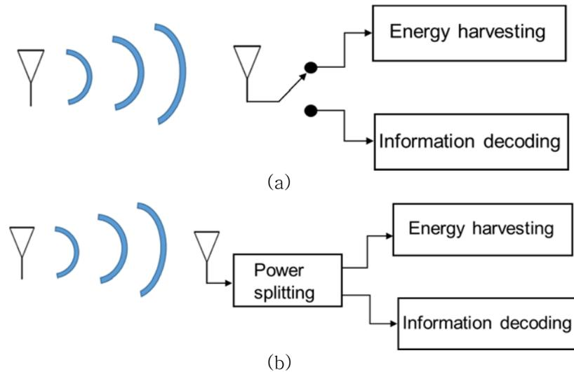
Fig. 1. Scheme of receiver operation in SWIPT (a) Time switching (b) Power splitting
