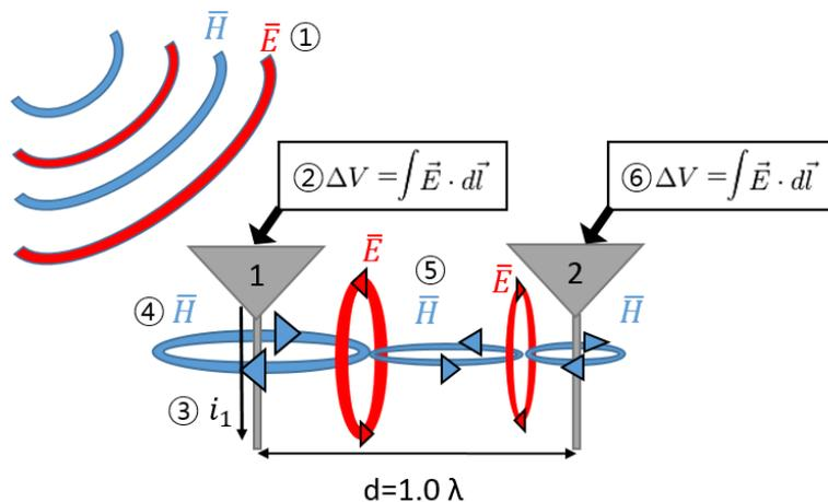
Fig. 2. Electromagnetic coupling between antennas.
