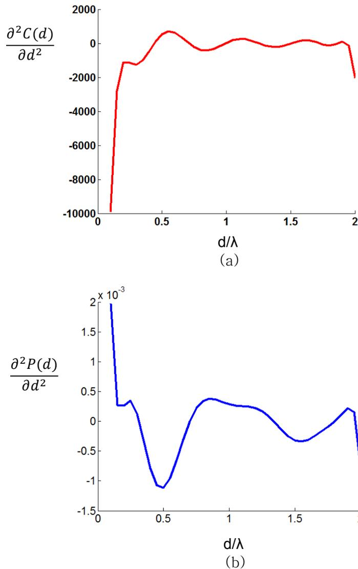
Fig. 18. Results of Hessian operation: (a) For channel capacity (b) For Received power.
