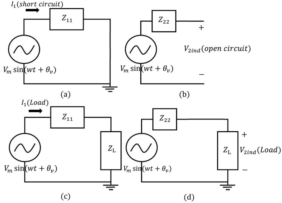
Fig. 4. Circuit models of (a) dipole antenna 1 (short circuit) (b) dipole antenna 2 (open circuit) (c) dipole antenna 1 (Load is connected) (d) dipole antenna 2 (Load is connected).
