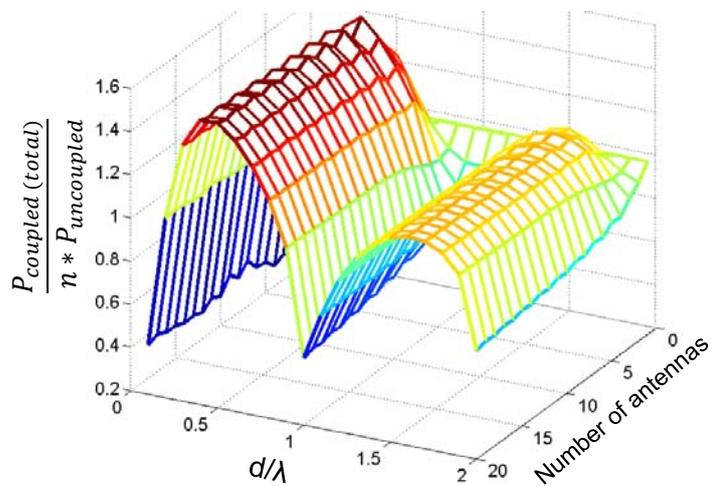
Fig. 15. The ratio of the coupled case and uncoupled case: depending on the number and spacing of antenna.
