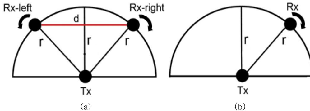
Fig. 7. Comparison of (a) coupled and (b) uncoupled case.  $d$  is the distance between receiving antennas, and  $r$  is the distance between Tx and Rx.
