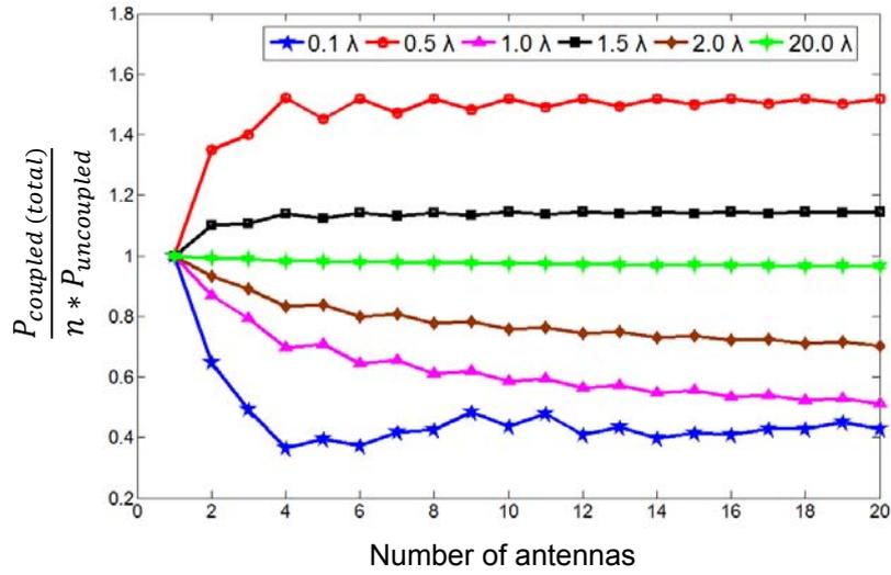
Fig. 13. Analytical results of power gains of the coupled case depending on the number and spacing of antenna.
