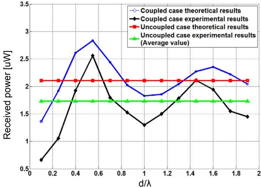
Fig. 9. Per-antenna received power of dipole antennas.
