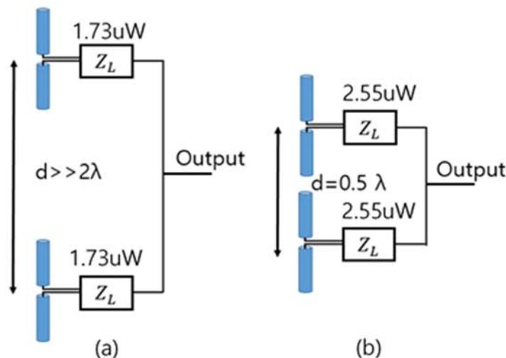
Fig. 10. The received power of dipole antenna: (a) the uncoupled case (b) the coupled case with mutual coupling increasing the received power.
