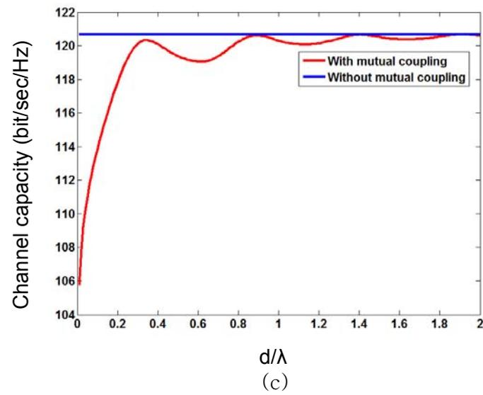
Fig. 17 The channel capacity with spacing of antennas : (a) Rx=2 (b) Rx=3 (c) Rx=4
