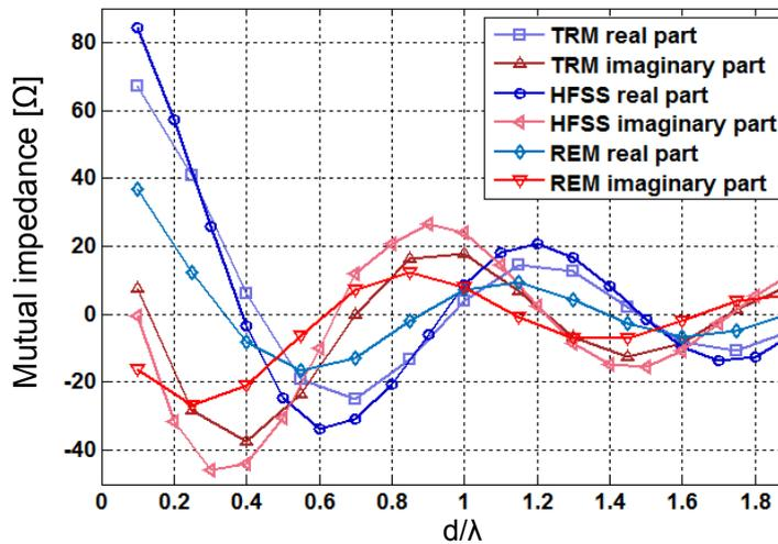
Fig. 5. Comparison of transmitting and receiving mutual impedances.
