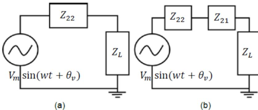
Fig. 6. Equivalent circuits of dipole antenna 2 with input impedance  $Z_{22}$ , mutual impedance  $Z_{21}$ , load impedance  $Z_L$  and applied voltage  $V_m$ : (a) uncoupled case (b) coupled
