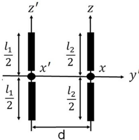
Fig. 3. Two half wavelength dipole antenna array (side by side).
