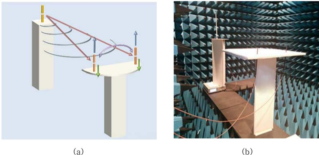
Fig. 8. Experiment setup: (a) Scheme of two dipole array experiments (b) Picture of the low frequency anechoic chamber.
