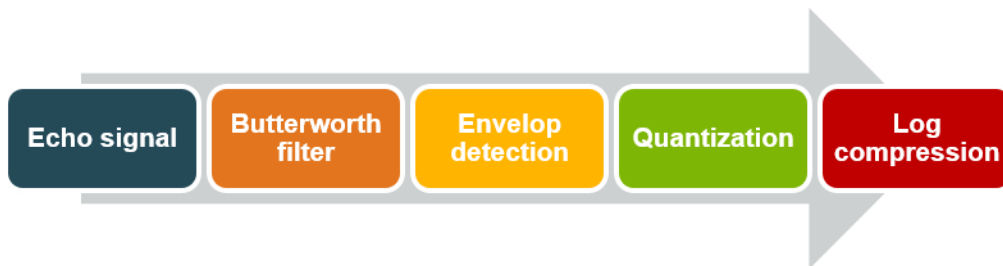
Figure 12. Siquence of the ultrasound image reconstruction.
