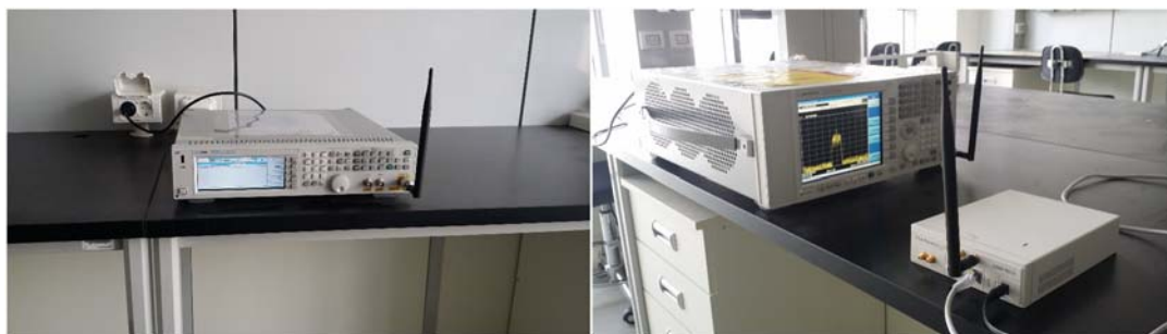
(b) N5182A MXG Signal Generator
