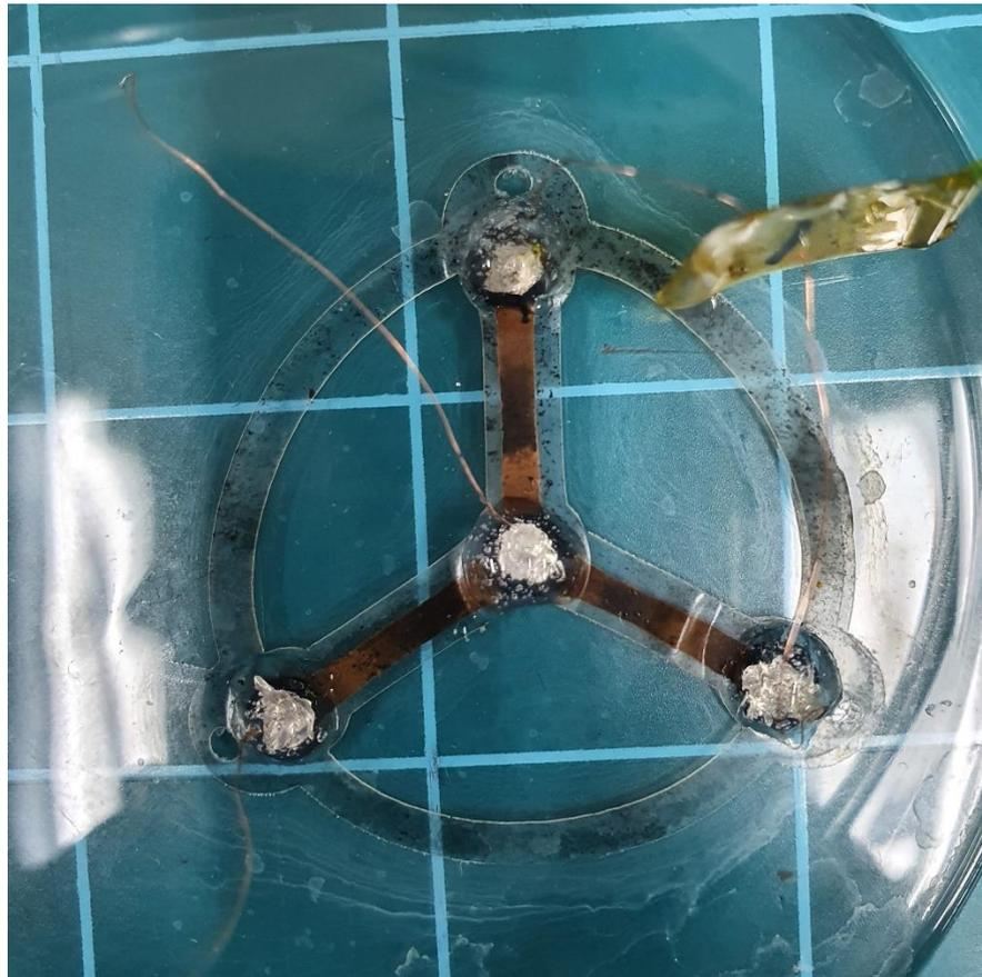
**Figure 18.** The fabricated 3-channel strain sensor.
