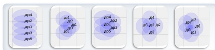
Figure 9. Types of topologies used in the simulation. We use five topologies consisting of five nodes with UAV modeling applied. The topology shapes used, from left to right, are linear, v-shaped, trapezoid, star, and pentagon.
