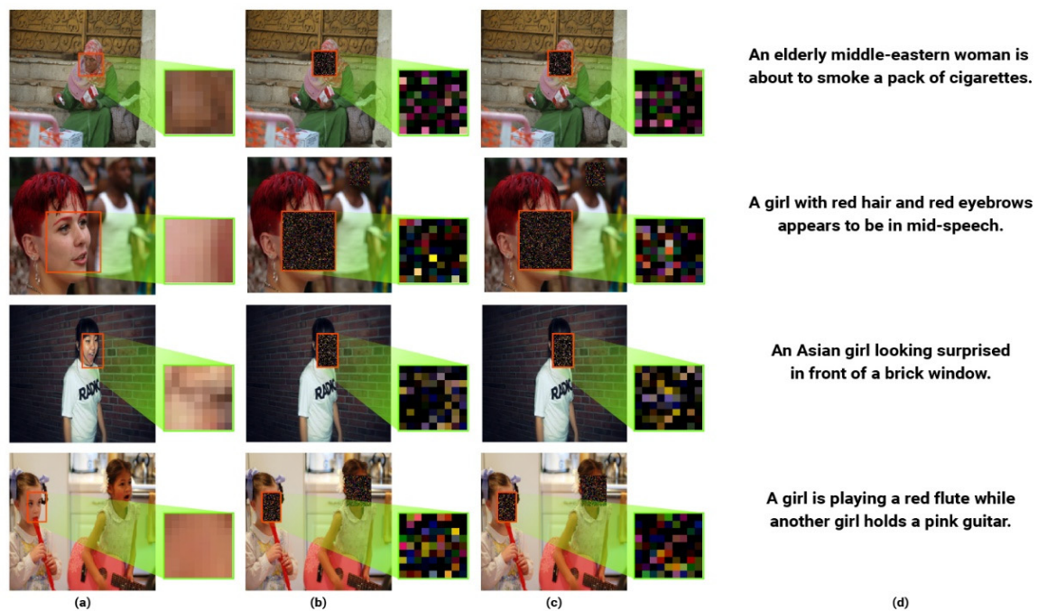
Figure 2. Illustration of partially encrypted images using DRPE. (a) Original image from the dataset, (b) partially encrypted images with the real part of the encrypted region of interest using DRPE, (c) partially encrypted images with the imaginary part of the encrypted region of interest using DRPE, and (d) the corresponding caption of the original image. The red boxes are the manually selected sensitive regions of interest in the original images and the encrypted regions in the partially encrypted images. The green boxes are the 9 \times 9 center matrix of the selected regions.
