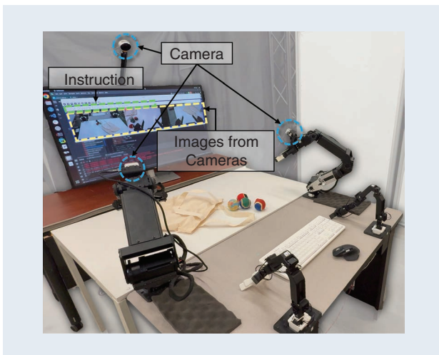
FIGURE 7. Example of data collection setup using PAPRLE.
