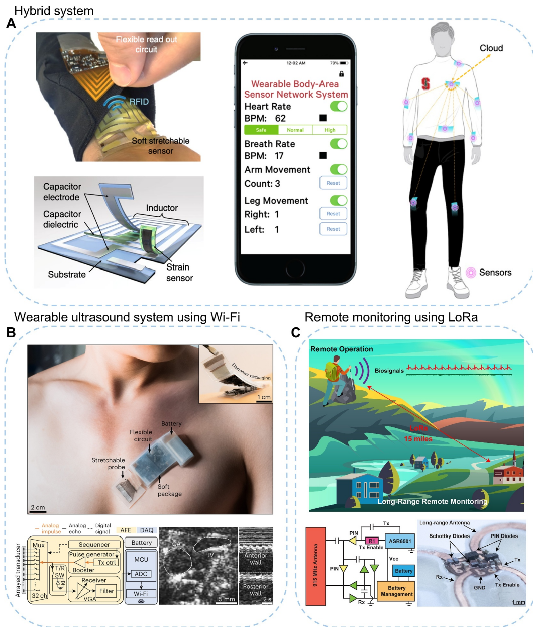
FIGURE 3 | Hybrid and other wireless communication technologies. (A) Wireless body-area sensor network based on stretchable passive RF tags and a BLE-enabled reader module. Reproduced from our previous work. [32]. Copyright 2019, Springer Nature. (B) Fully integrated wearable ultrasound system that uses wireless phased arrays on the skin and Wi-Fi for high-bandwidth deep-tissue monitoring in freely moving subjects. Reproduced with permission from Ref. [33]. Copyright 2023, Springer Nature. (C) Biosymbiotic platform for chronic, long-range monitoring of biosignals in limited-resource settings using low-power wide-area network connectivity. Reproduced with permission from Ref. [34]. Copyright 2023, The Author(s).
